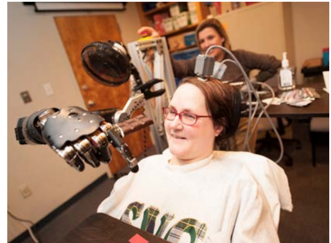
Figure 2. Jan controls a robotic arm by thinking about bringing the chocolate to her mouth. (photo credit: UPMC)
