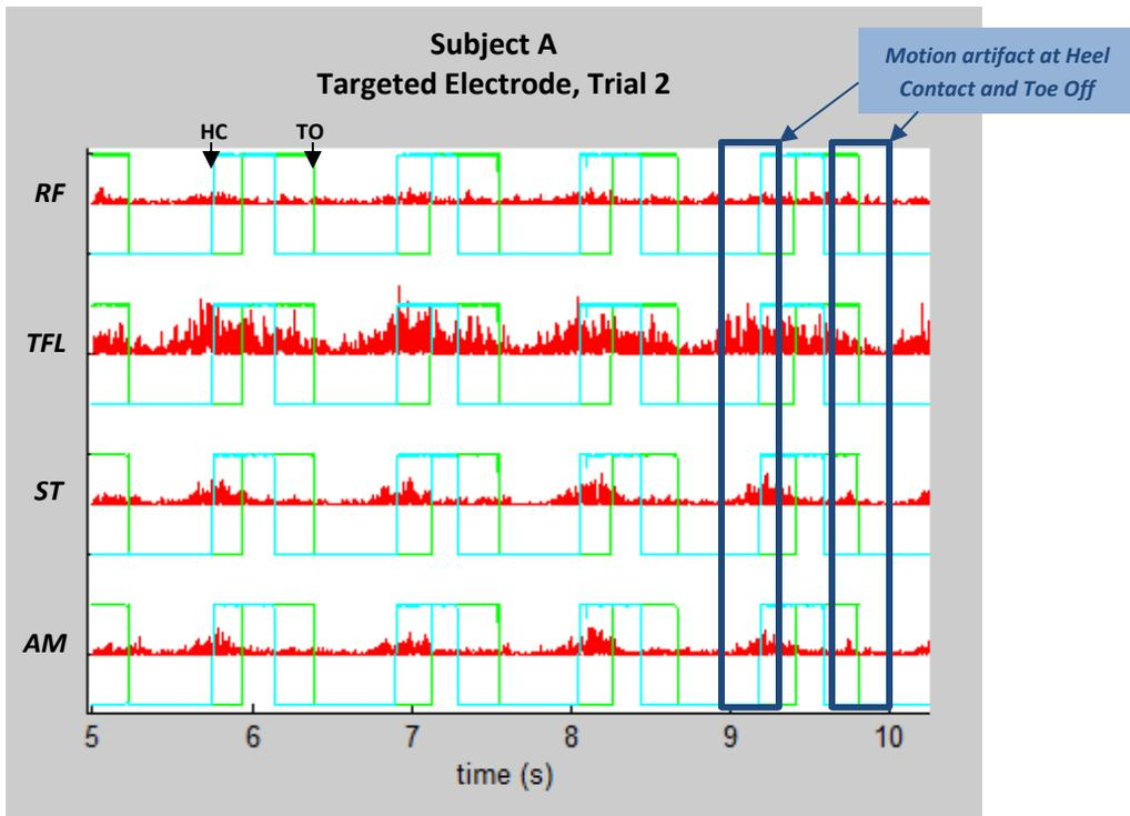
Figure 5. Trial #2 data for Subject A using the MyoWare Targeted Electrodes.
