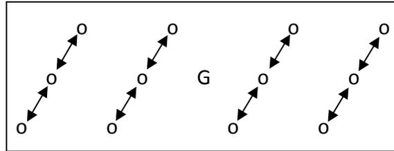
Figure 2. Configuration for Grid electrode placement in gel liner.
