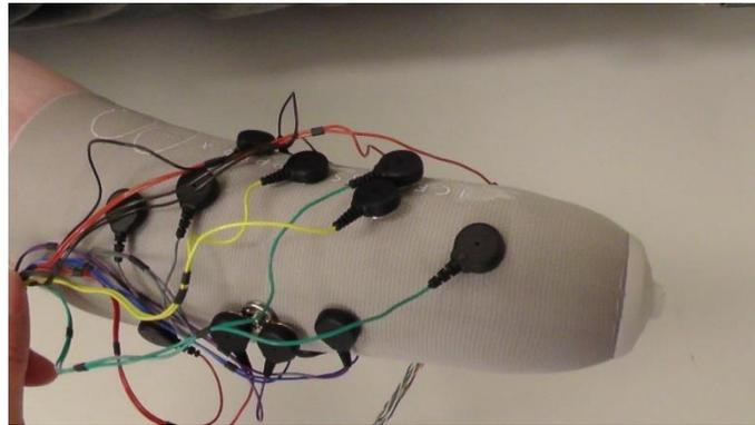
Figure 3: Silicone liner with PR electrode and snaps connected.
