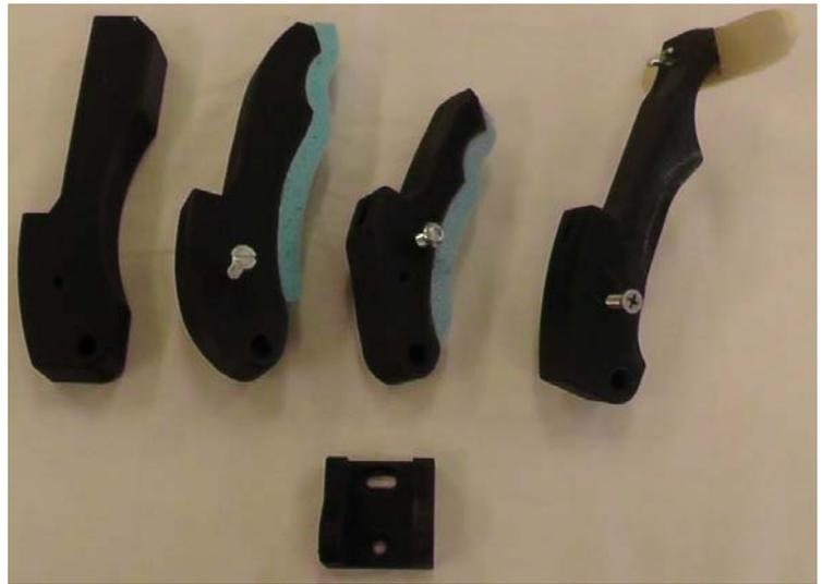
Figure 2: Design iterations of thumb from initial block design (left) to final design with added cross point (right).
