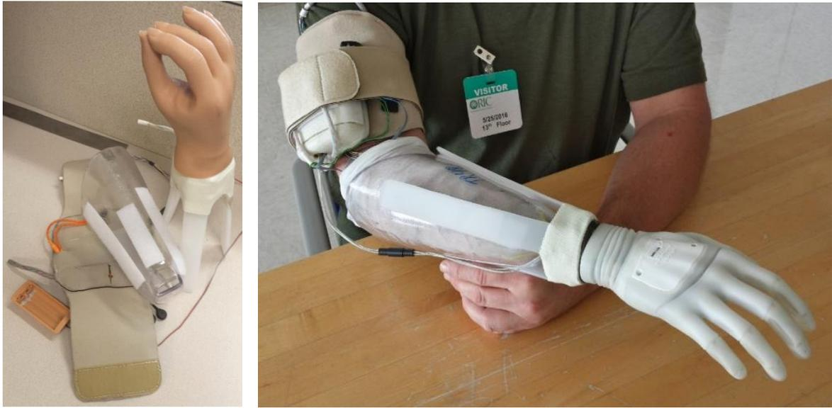
Figure 1: *Left* Quick interchange suspension interface for attaching the hand to the wrist and socket.
